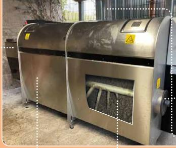
The first chamber is where composting takes place, while the second chamber is for ripening.
