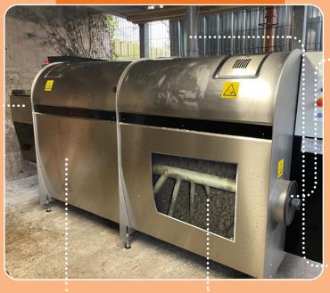
The first chamber is where composting takes place, while the second chamber is for ripening.
